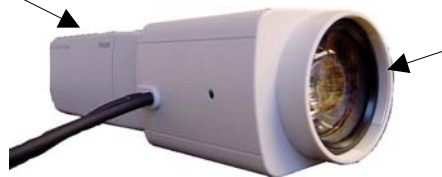
Camera with assembled motorized zoomlens.
